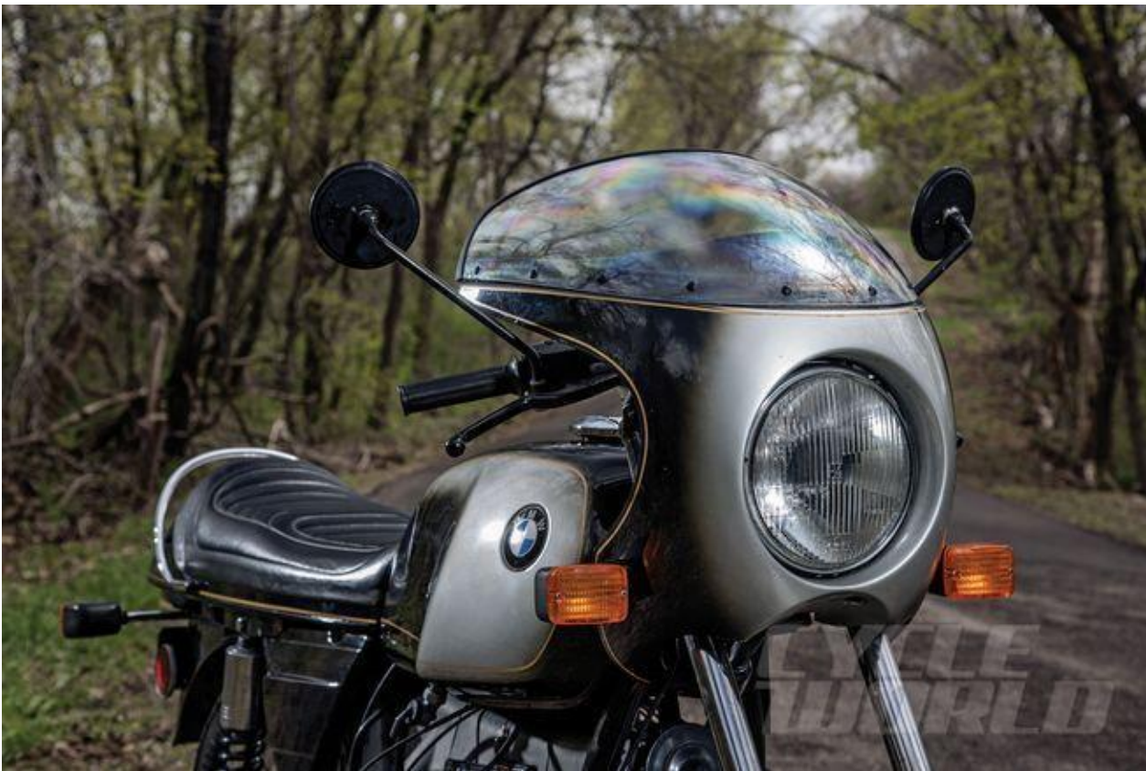
Photo #7 - A café fairing makes high-speed touring considerably more serene and easy on the arms and back.- Marc Urbano
