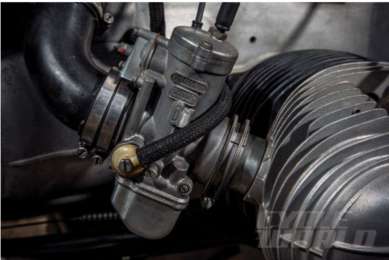
Photo #10 - Dell'Orto pumper carbs give the R90S immediate, Ducati-like throttle response.
