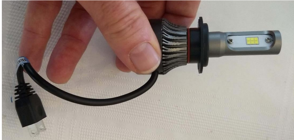
Figure 5: ODX S6 6000 Lumen LED
