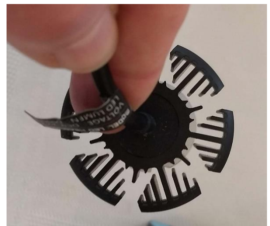
Figure 4: ODX V3 3000 heatsink
