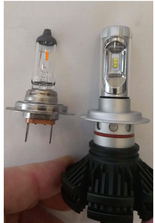
Figure 3: H7 Halogen vs ODX V3 3000
